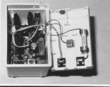
Photo 3 – mains plug-box with Receiver unit installed
