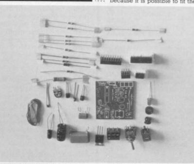
Photo 2 - the Receiver kit before construction
